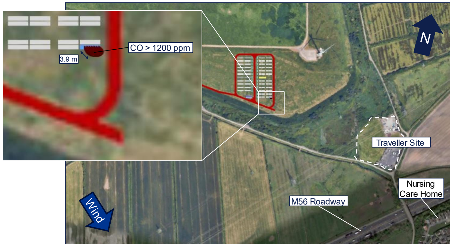
Figure A 6: Case 102 – Carbon Monoxide Plot with Wind from NW at 10 m/s
